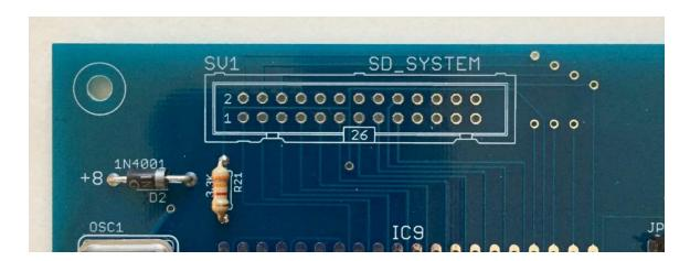
All of the even numbered pins are on row closest to the top edge of the circuit board while all the odd numbered pins are on the other row.
